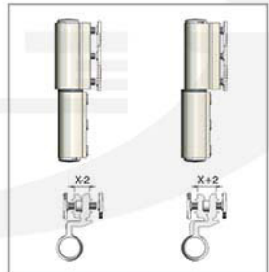
Side adjustment typical of conventional clamp-fixed hinges
